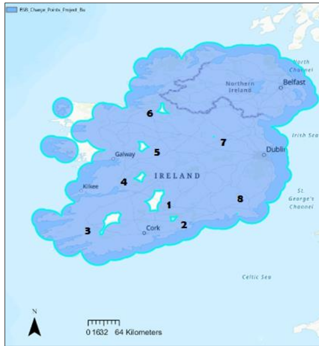
Figure 16 Buffer ring analysis of public charging network assuming an effective driving distance of 52km. Source: ESNB
