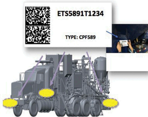
Figure 15. Sample Barcode on the asset at eye level and possible locations (Author).
