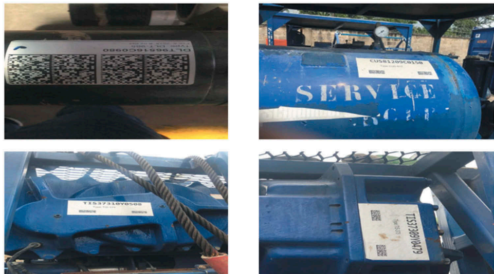
Figure 16. Sample Barcode on the asset at eye level and possible locations (Author).
