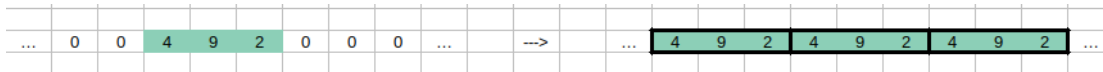
Figure 3: Example of periodic summation of a zero-padded finite sequence where the period equals to the sequence length ( N = \tilde{N} ).
