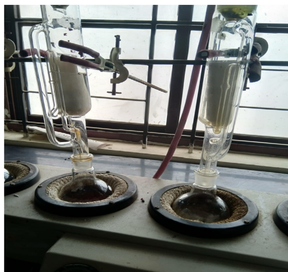
Fig. 1. Extraction of algae setup.
