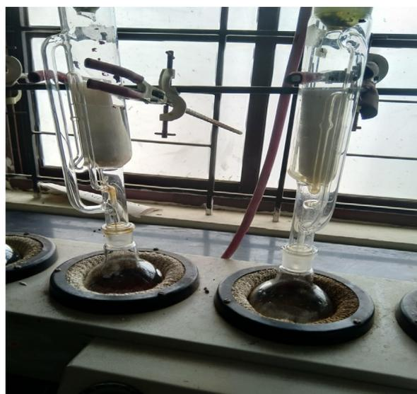
Fig. 1. Extraction of algae setup.
