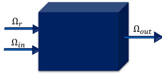
Fig. 5. Black box model based on the energy level equilibrium in the heating furnace.
