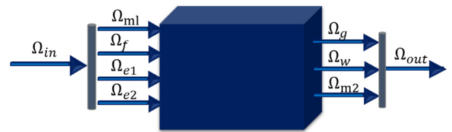
Fig. 3. Black box energy level analysis model of the oil transfer station subsystem.
