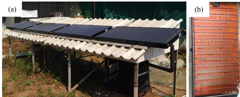
Fig. 3. (a): Tested unglazed PVT modules and (b) back of module without insulation.
