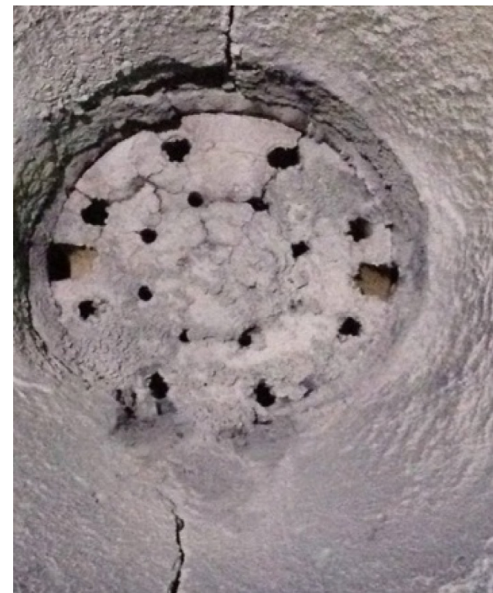
Fig. 2. The fused burner holes.
