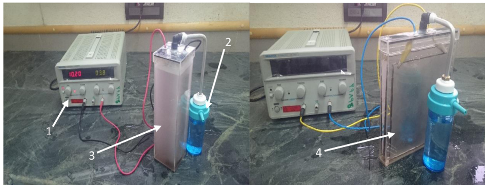
Fig. 2. Different electrolysis chambers for cylindrical and flat plate electrodes experiments.
