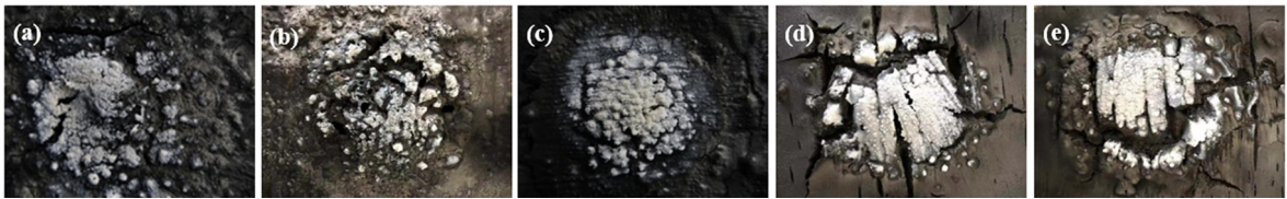
Fig. 2. The residual carbon photographs of coatings after fire test.
