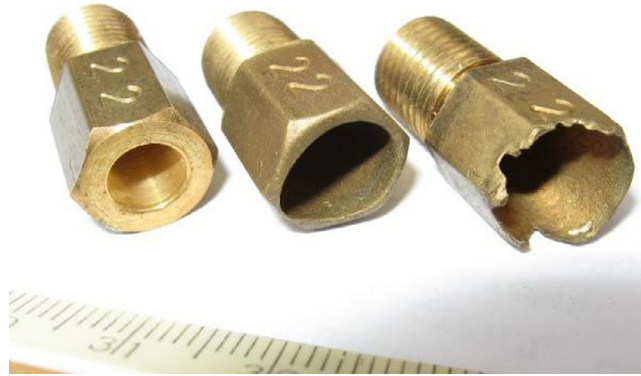
Fig. 4. Cavitation erosion inside bronze nozzles.
