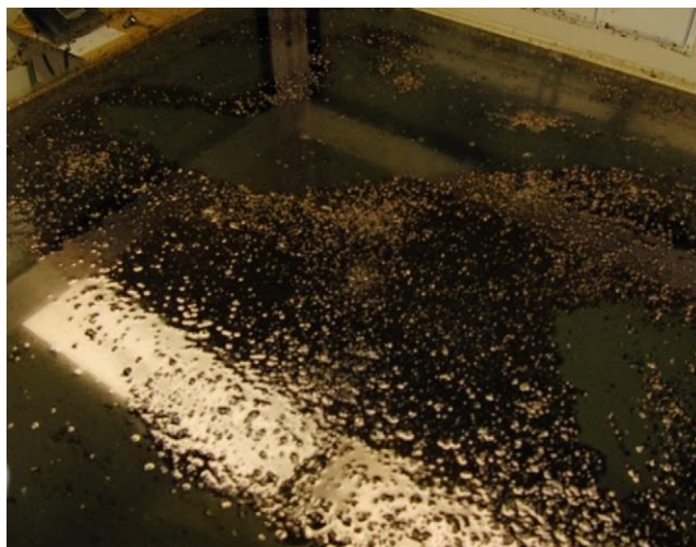
Fig. 7. Separated bitumen on the surface of the tank.
