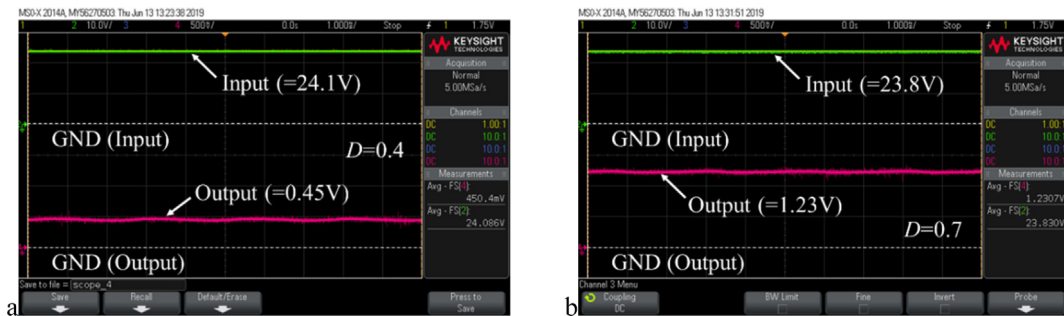
Fig. 4. Measured output voltage: (a) D = 0.4 V; (b) D = 0.7 V.
