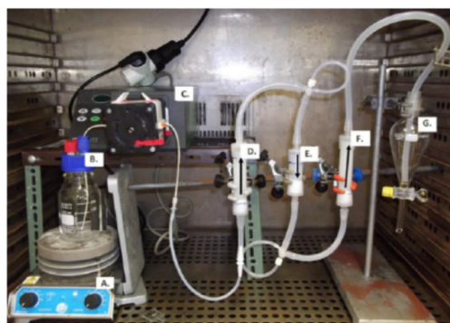
Fig. 1. Experimental setup for the continuous-regime experiment. A — stirring device; B — Feed mixture; C — Pump for reactional mixture feeding; D — 1st fixed bed bioreactor; E — Resin column; F — 2nd fixed bed bioreactor; G — Sampling point.
