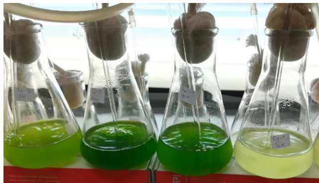
Fig. 6. Cultures of microalgae Chlorella vulgaris in 250 mL flasks for the nitrate nutritional stress (from the left flasks include trials of C1, C2, C2 and C3).
