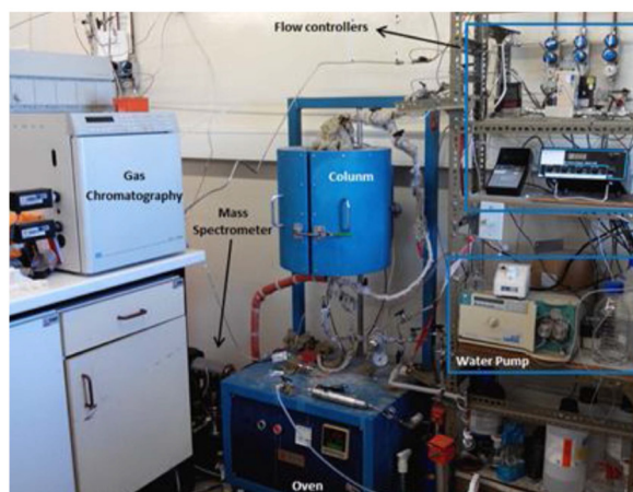
Fig. 1. Reactor setup used for BMR experiments.
