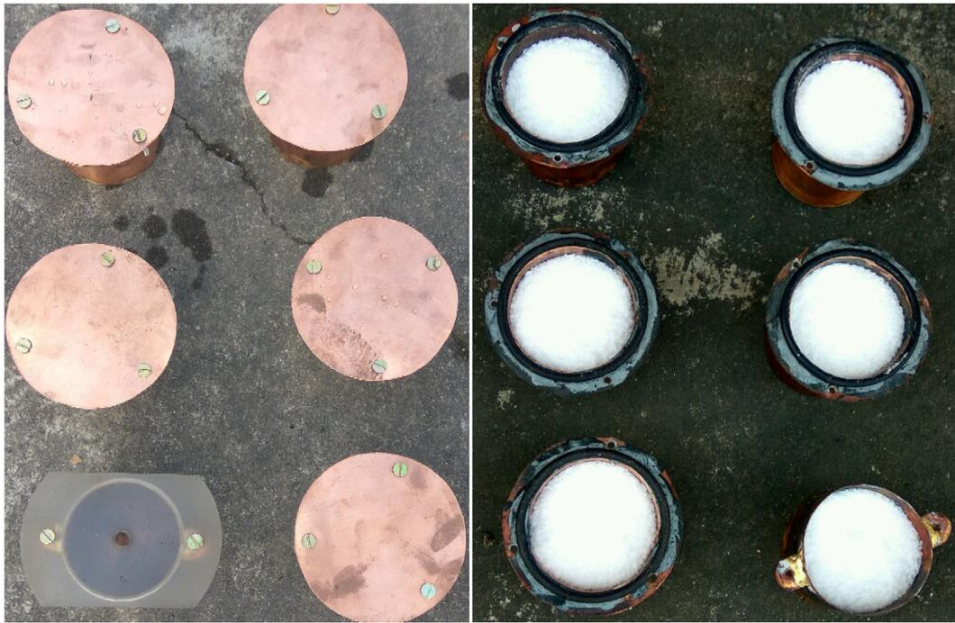
Fig. 3. Pictorial view of PCM loaded copper cylinders.
