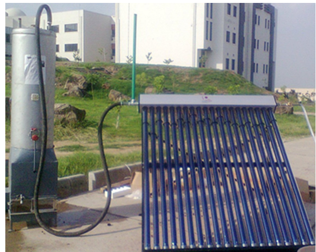
Fig. 5. Experimental set-up: heat pipe evacuated tube manipulate connected to the hot water storage tank and multi-fuel furnace.
