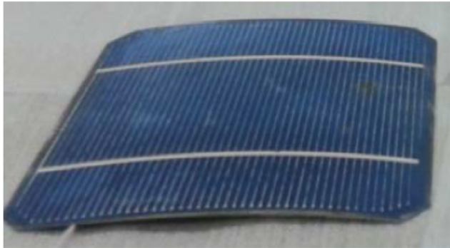
Fig. 10. Screen printed finished type Si wafer.
