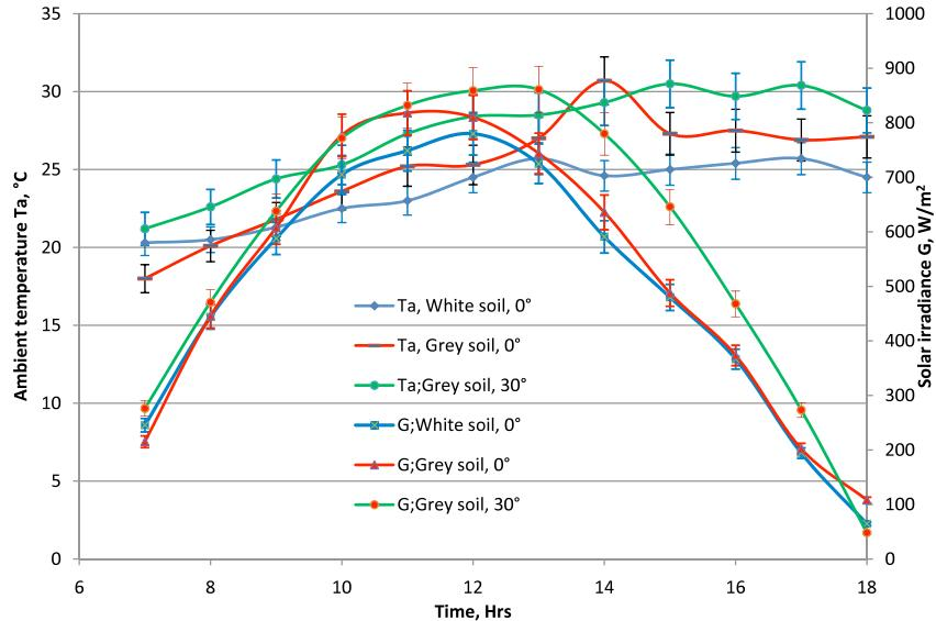
**Fig. 2.** Variation of the solar irradiance and ambient temperature with time.
