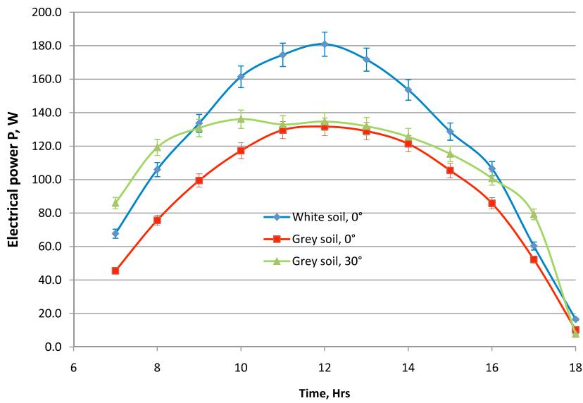
**Fig. 4.** Electrical power of the PV system.
