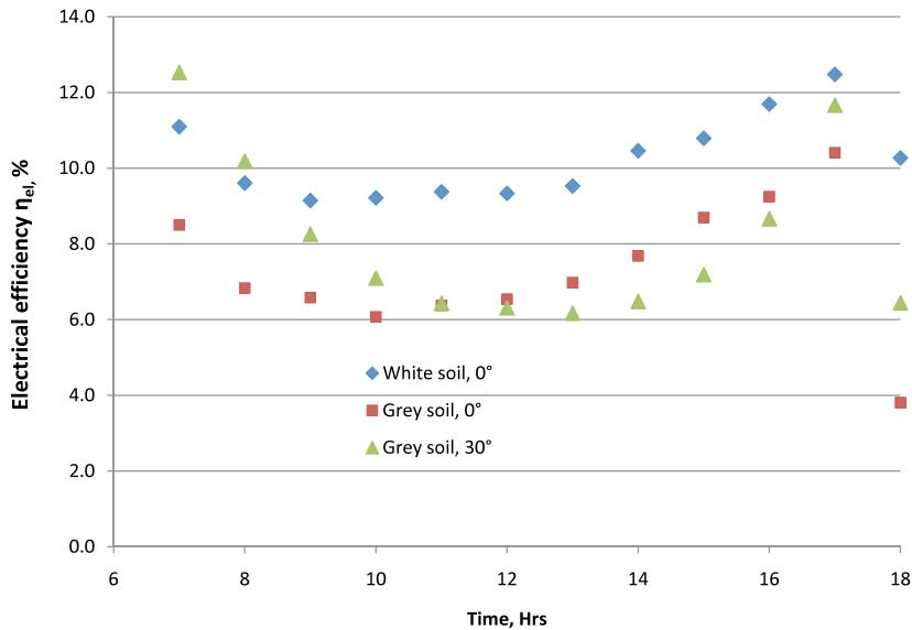
**Fig. 5.** Electrical efficiency of the PV system.
