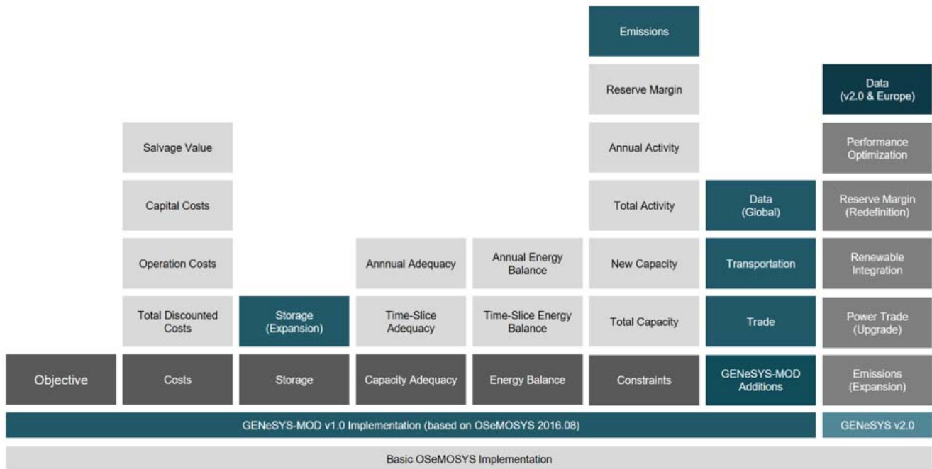
Figure 2: Technical block structure of GENeSYS-MOD v2.0. The grey boxes in darker shade on the right side represent changes and additions made to previous versions. Based on Howells et al. (2011).
