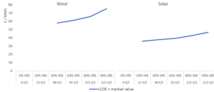
Figure 10: Market values for wind power and solar PV and levelized costs of electricity for increasing VRE shares driven by CO 2 pricing in a stylized German setting.
