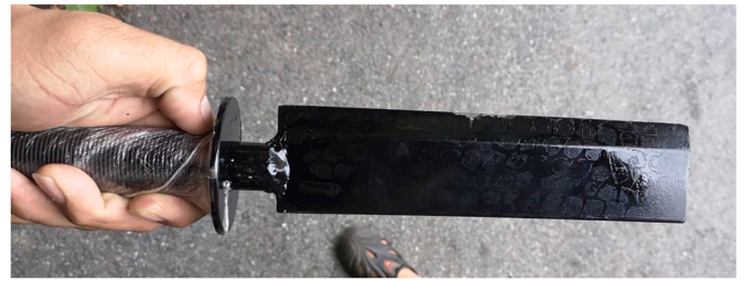
Fig. 6. Optimal knife design (handle in side position, 9 inch blade, thick blade, guard).
