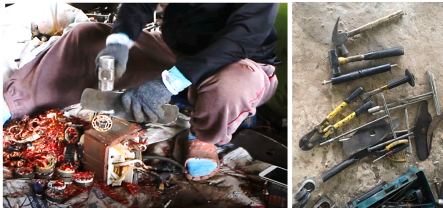
Fig. 1. E-waste worker dismantling a stator with a blade and hammer (left). Set of typical tools used to dismantle E-waste (right).
