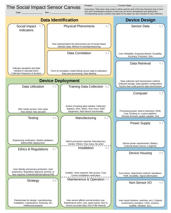
Fig. 1. The Social Impact Sensor Canvas for guiding the development of sensor systems used to measure the social impacts of products in developing countries.
