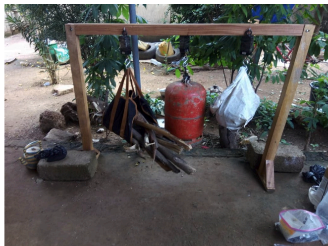
Fig. 3. FUEL installation for (from left to right): wood, LPG, and charcoal, Burkina Faso.
