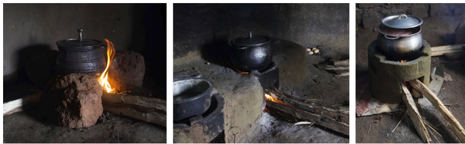
Fig. 2. Stove Models (from left to right): Three Stone Fire, Locally Mudded Stove, Rural Wood Stove, Uganda.
