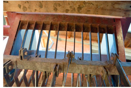
Fig. 5. Self-produced chestnut deburring machine.
