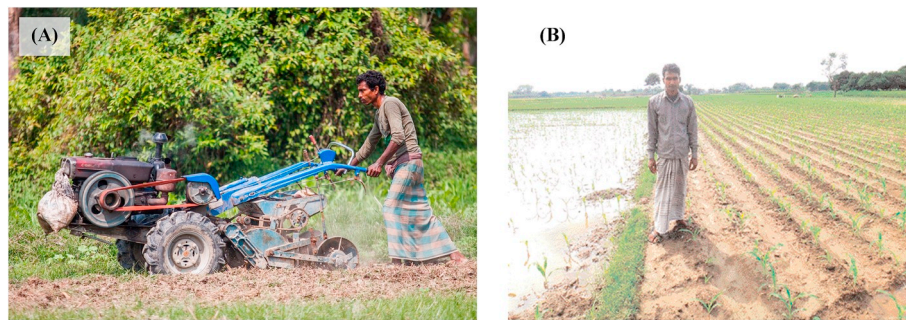
Fig. 1. (A) Two-wheeled tractor with an attachable bed planter in Bangladesh (courtesy Ranak Martin). (B) Bed planted maize (right) compared to flat planted and waterlogged maize (left) following a storm event Bangladesh (photo from Krupnik et al., 2013).
