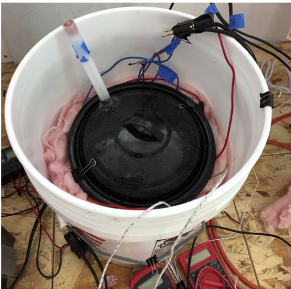
Fig. 4. Each solar panel powered a different heating technology in three insulated cook pots made of 4-quart steel pots insulated with pink fiberglass insulation around the perimeter and below (but not above), containing 3 L of water. (For interpretation of the references to colour in this figure legend, the reader is referred to the Web version of this article.)
