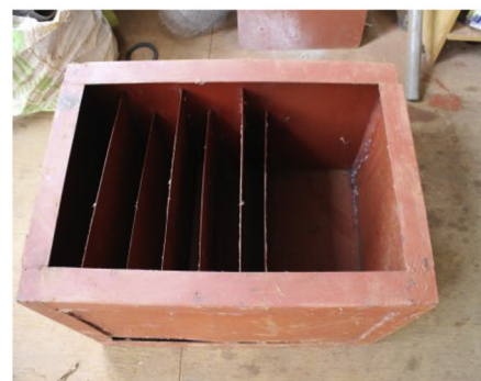
(b) Anaerobic baffled reactor.
