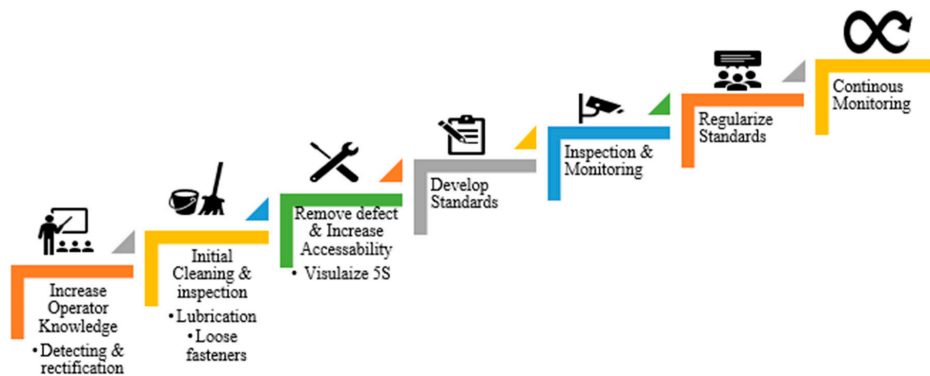
Figure 12. Autonomous maintenance procedure.
