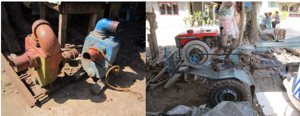
Figure 1A-93. The STWs use 3x3 self-priming centrifugal pumps (left) and 7 Hp Kubota engine (right)
