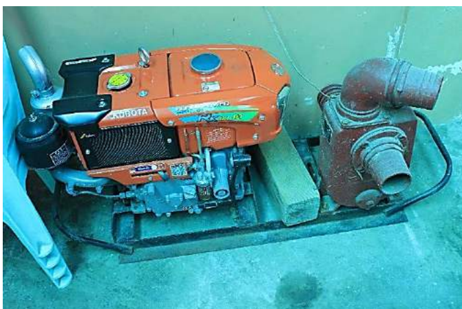
Figure 1A-12. A typical pumpset with a 4x4 self-priming centrifugal pump driven by an 8-Hp Kubota diesel engine (RK80-1S)
