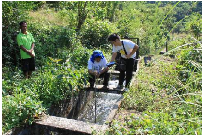
Figure 1A-41. Measuring discharge at the main canal during the walkthrough
