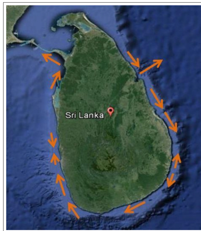
Figure 9: Near-Shore Sediment Transportation Directions
