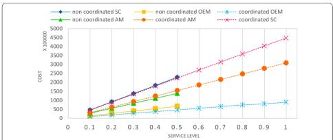
**Fig. 3** The differences between the costs of OEM, AM, and the supply chain in two scenarios for different service levels. *Note*: For the service levels more than 0.5, the problem is infeasible for the non-coordinated scenario, that is, infinity costs
