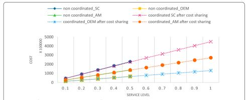
**Fig. 4** The differences between the costs of OEM, AM, and the supply chain in the non-coordinated scenario and the coordinated scenario after applying the cost-sharing mechanism. Note: For the service levels more than 0.5, the problem is infeasible for the non-coordinated scenario, that is, infinity costs)
