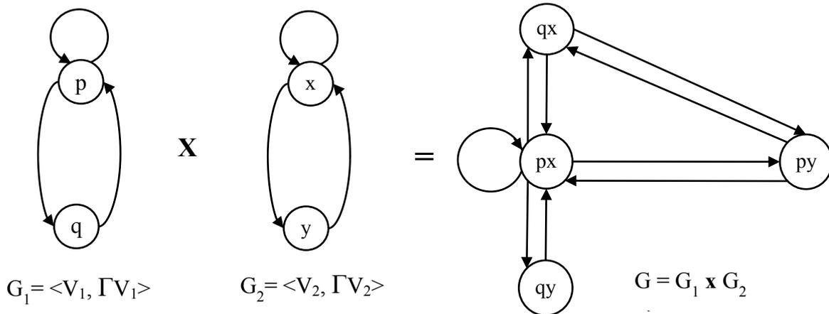
Figure 3. Potential dynamics of a two-buffer object represented by the vertices  $V_1$  and  $V_2$  of the graphs  $G_1$  and  $G_2$ , written in the form of a Cartesian product  $G_1 \times G_2$ , where the symbol  $\times$  written in bold type indicates the Cartesian product of the two reproduced sets  $G_1$  and  $G_2$  (Source: Authors own research)
