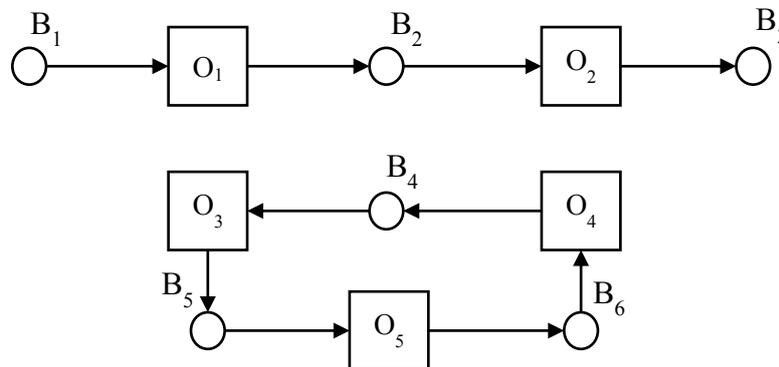
Figure 1. Chain of two objects and a loop of three two-buffer objects, where the buffers  $B_2$ ,  $B_3$ ,  $B_4$ ,  $B_5$  and  $B_6$  are the proper buffers for the objects  $O_1$ ,  $O_2$ ,  $O_4$ ,  $O_3$  and  $O_5$
