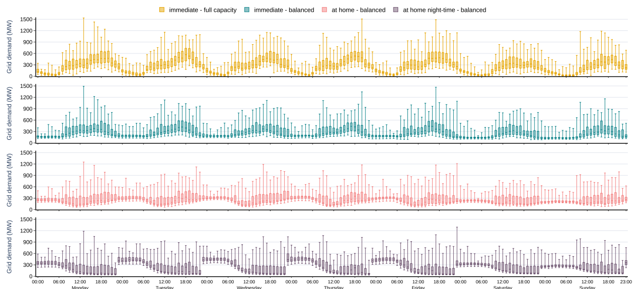
Fig. 6 Simulated grid electricity demand time series for a fleet of one million BEV for four charging strategies, summarized in box plots for each hour of the week.
