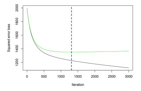
Note: Green line = squared error loss for the test data obtained by means of five-fold cross-validation. Black line = squared error loss computed for the estimation data. Dashed vertical line = optimal number of trees. Learning rate = 0.005. Test and training data were obtained by 5-fold cross-validation, minimum number of observations per terminal node = 10. Tree size = 5. Boosting proportion = 0.5.
