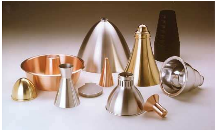
Fig. 2. Typical workpieces of shear forming, see Ott [1]
