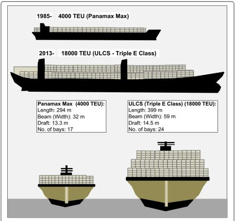
**Fig. 7** Overview of the scale of container ships used along the given line shipping trunk line/route (AECOM 2012; Rodrigue et al. 2017; PR 2011)
