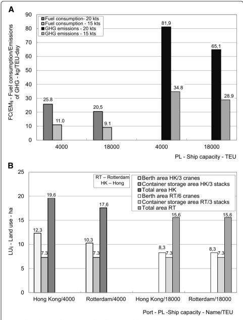
**Fig. 11** The indicators of environmental performances of the trunk line/route. a Fuel consumption and emissions of GHG. b) Land use
