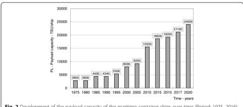
**Fig. 2** Development of the payload capacity of the maritime container ships over time (Period: 1975–2016) (Rodrigue et al. 2017; ITF 2015; UNCTAD 2017)
