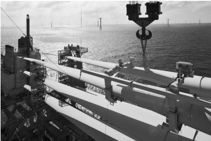
Figure 6: Transport frame for turbine blades on a heavy-lift vessel (Image: Servion)
