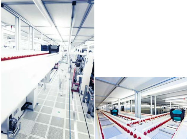
Figure 3: Part of the conveyor AHMS – depicting open carrier transportation on top left (Courtesy of Infineon Technologies Dresden GmbH)
