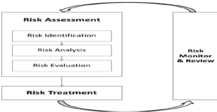
Figure 2 General Risk Management Process adapted from Jenkins et al., (2010) and Rao and Goldsby (2009)
