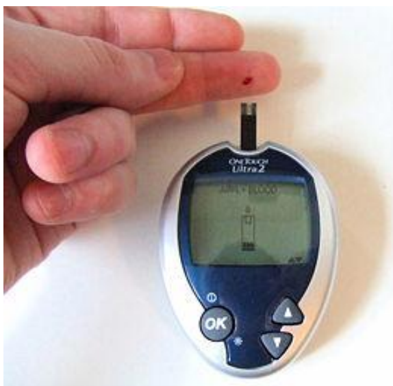
Figure IV-3. A blood glucose meter (OneTouch Ultra2 from LifeScan; a company in the Johnson & Johnson group). A drop of blood is transferred to a test strip, which has been inserted in the device.
