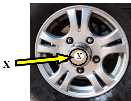
Fig. 3 Alloy wheel in assembly, X = center hole diameter of \phi 50.000^{(\pm 0.050)}
