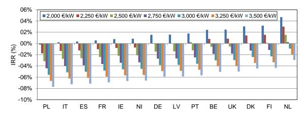
Figure 6: Impact of technology cost variations on the IRR of wind offshore investments across Europe, 2030
