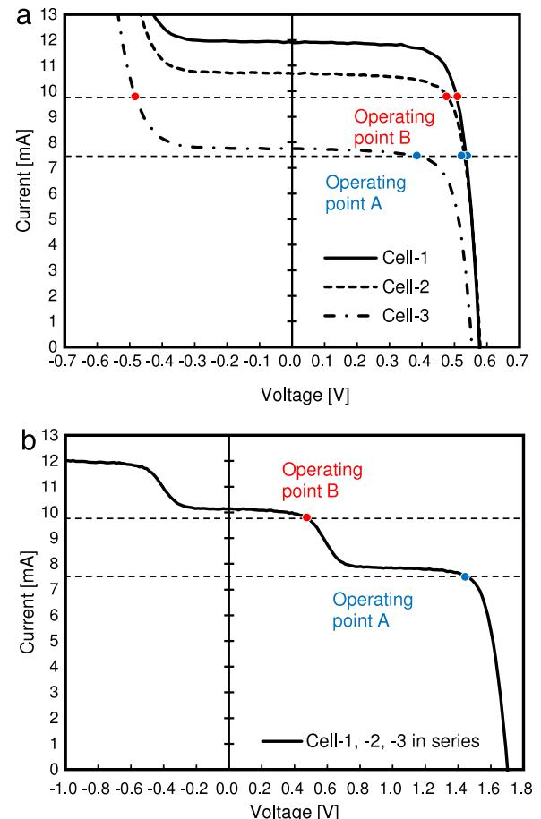
**Fig. 1.** Typical current–voltage ( $I$ – $V$ ) characteristics under standard air mass 1.5 (AM 1.5) solar spectrum light: (a) cells with different compositions and (b) a module comprising the serial connection of the cells shown in (a).
