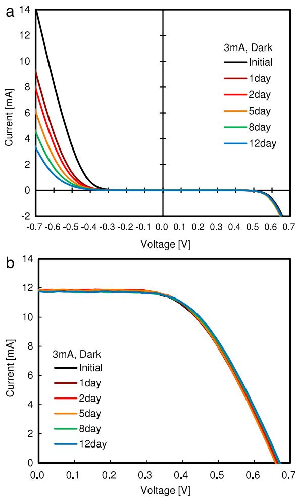
**Fig. 2.**  $I$ - $V$  characteristics of dye-sensitized solar cells (DSSCs) through which a constant forward current of  $3\text{ mA}/\text{cm}^2$  has been flowed: (a) in the dark and (b) under standard AM 1.5 global sunlight.
