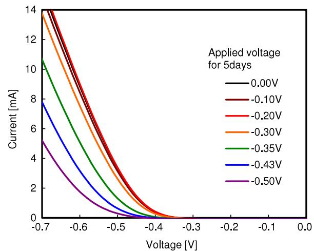
**Fig. 3.**  $I$ - $V$  characteristics of DSSCs to which constant reverse voltages have been applied for 5 days in the dark.
