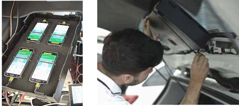
Figure 2: Measuring cases with cell phones (left) are mounted in windows of drive test car (right).
