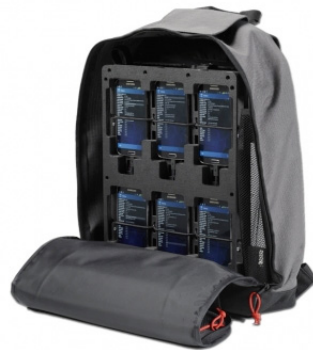
Figure 5: Carrying case with mountings for multiple cell phones
