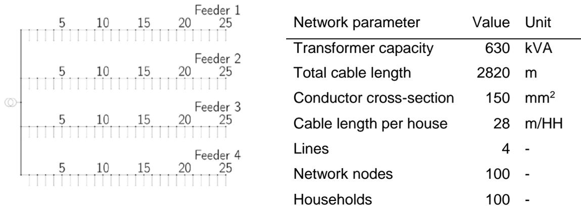
Figure 2: Topology of the suburban network and network parameters for 2030
