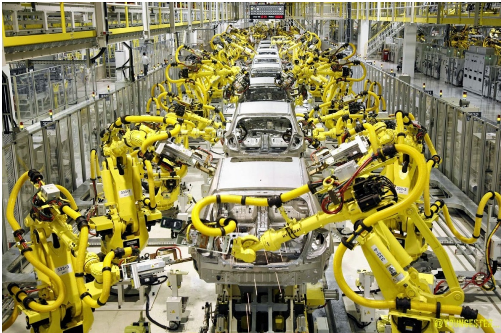
Figure 9. An assembly line of cars made up exclusively of industrial robots (source: Magazyn Przemysłowy, 2015)
