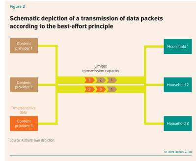
The time-sensitive data packet has to wait until transmission capacities are available: Households loose the potential additional benefit of the time-sensitive service.
