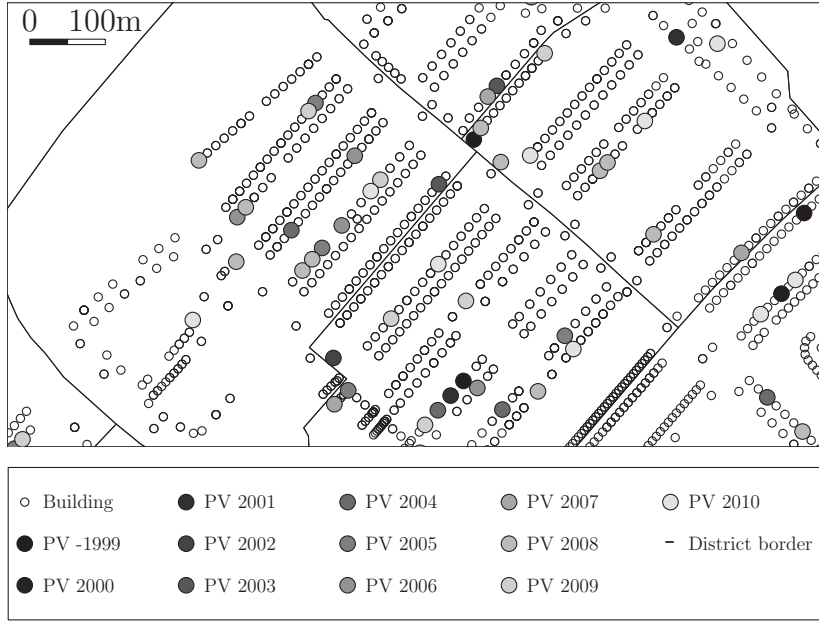
Figure 2: Example of the PV adoption process. Hollow circles represent potential adopters. Filled circles are PV installations. Newer PV installations are colored in light gray.
