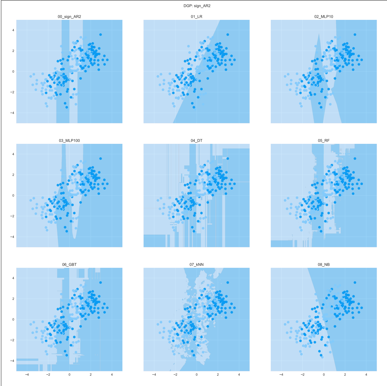
Figure 3: Decision boundaries obtained for SAR(2) process. The lighter shaded areas indicate a forecast value of “1”, i.e., \hat{s}_t is larger than or equal to s_{t-1} ; the darker shaded areas a forecast value of “0”. The x-axis denotes s_{t-1} , the y-axis s_{t-2} . The dots represent a subset of the actual observations that were used to fit the models with the color coding being similar to the one of the areas.
