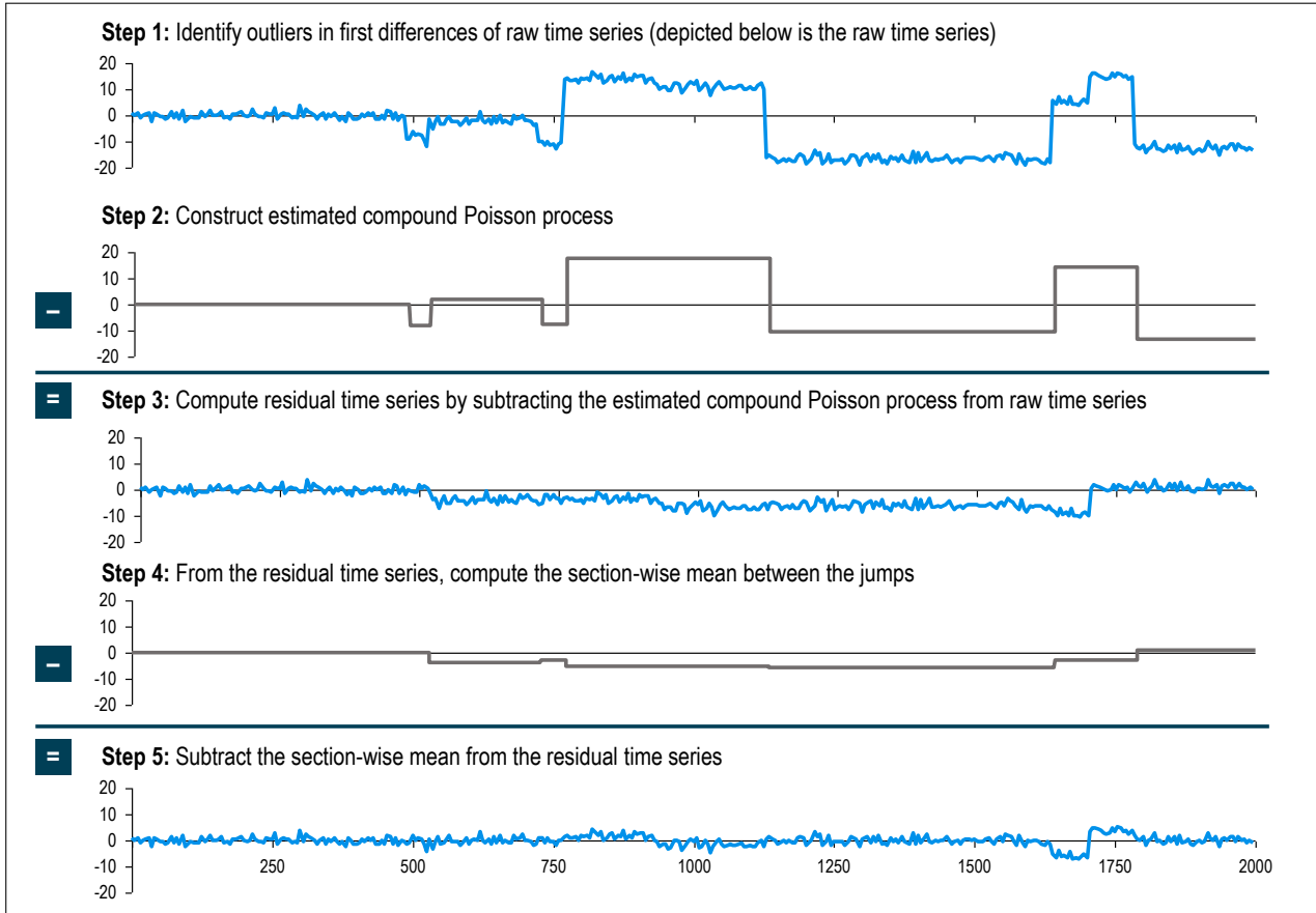
Figure 1: Procedure to remove jumps with LOF.
