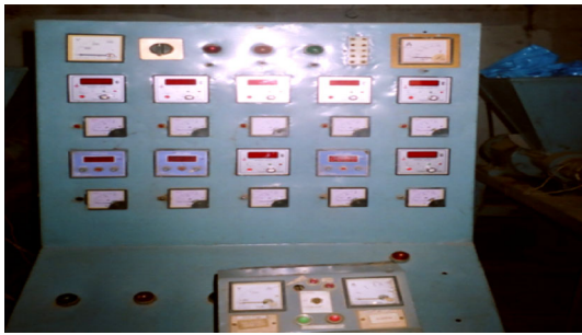
Fig. 5 Panel board showing different zone temperatures
